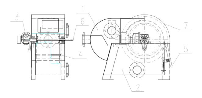
Supply tank (1) captures the stream of supplied water and allows uniform flow on the
